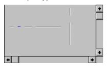
The first ULINE statement creates a horizontal line that covers one column. The hyphen in the first WRITE statement appears as a normal output field. The two hyphens of the second WRITE statement create a straight line that covers two columns. The next three hyphens together with the ULINE statement create a straight line that cover seven columns.
